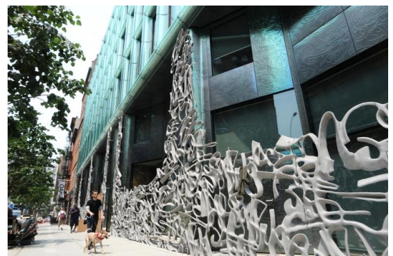
Fig. 4. Examples of art castings as the architectural decoration: a) the gate pattern; b) sections of aluminium castings of the collage, assembled along the large building in New York.
